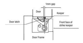
As drawn in the diagram above there should be a 1mm gap between the door latch and the front-face of the strike keeper, preventing the door from creating back pressure on the strike keeper when the door is closed.
